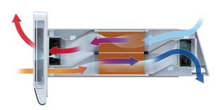
The regenerator is divided into two parts, which are isolated from one another, thus eliminating the transfer of heat and moisture between them. One of the fans operates in the supply mode: fresh cold intake air from outside flows through the first regenerator, and absorbs accumulated heat and humidity.
