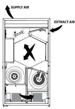
The unit is equipped with a recirculation damper. In recirculation mode it is opened and the supply and exhaust dampers are closed.
