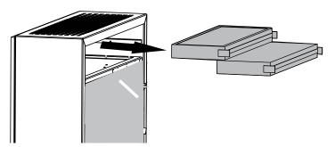
If an extract spigot is installed, remove the top protective panel and install the magnetic plug on the exhaust grille. When removing the panel, disconnect the grounding cable.
