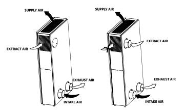
An additional extract spigot (Ø 100 mm) can be fitted to the unit to connect the exhaust air duct from additional premises, e.g. a bathroom. The spigot is included in the delivery set.
