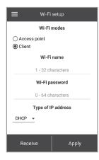
Access Point: access point mode without a home router. Up to 8 devices can be connected to the unit in this mode. Select the desired security level for the Access point mode: Open means no password protection. WPA PSK: password-protected. WPA2 PSK: password-protected. WPA/WPA2 PSK: password-protected (recommended).
