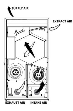
Warm stale extract air from the room flows to the unit, where it is filtered by the extract filter, then air flows through the heat exchanger and is exhausted outside by the extract fan.
