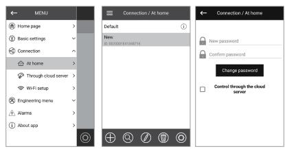
To manage the unit, create a new account. Open the mobile app and go to **MENU -> CONNECTION -> THROUGH CLOUD SERVER:**
