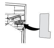
Lift the unit, insert the spigots into the corresponding air ducts installed in the wall.
