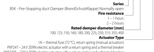
PKP230T – 230 V ZERN electric actuator with a return spring and a thermal breaker PVP24T – 24 V BELIMO electric actuator with a return spring and a thermal breaker PVP230T - 230 V BELIMO electric actuator with a return spring and a thermal breaker PSP24T – 24 V SIEMENS electric actuator with a return spring and a thermal breaker PSP230T – 230 V SIEMENS electric actuator with a return spring and a thermal breaker
