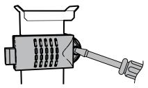
Fix the sensor in the exhaust air duct of the unit upstream of the heat exchanger. Connect the sensor connector to the connector with the cable of the control unit (installed by the manufacturer).
