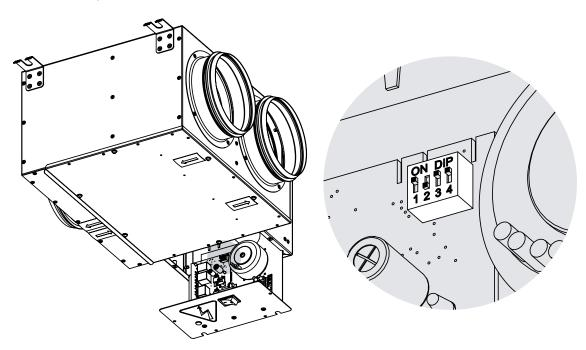
Using the table, select the desired running time and downtime of the fan for a period of 60 min and set the DIP switch levers to the appropriate position.
